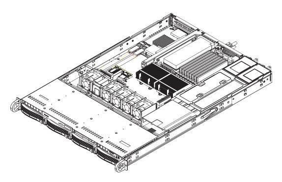
Figure 6-2. System Cooling Fans
